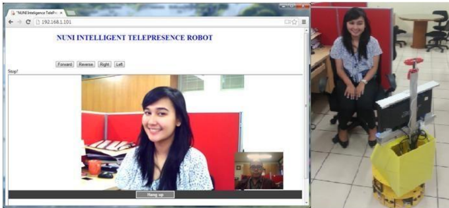
Figure 1.14 Intelligent Telepresence robot using omniwheel and controlled using Web [11].
